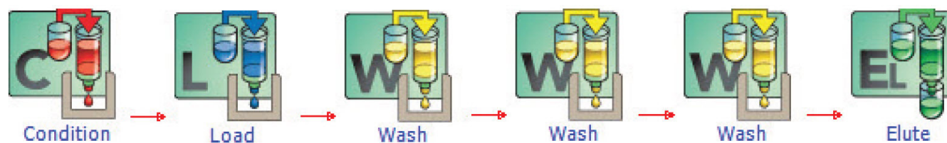
Figure 3 TRILUTION® LH Basic SPE Tasks for Solid Phase Extraction of Patulin from Apple Juice
