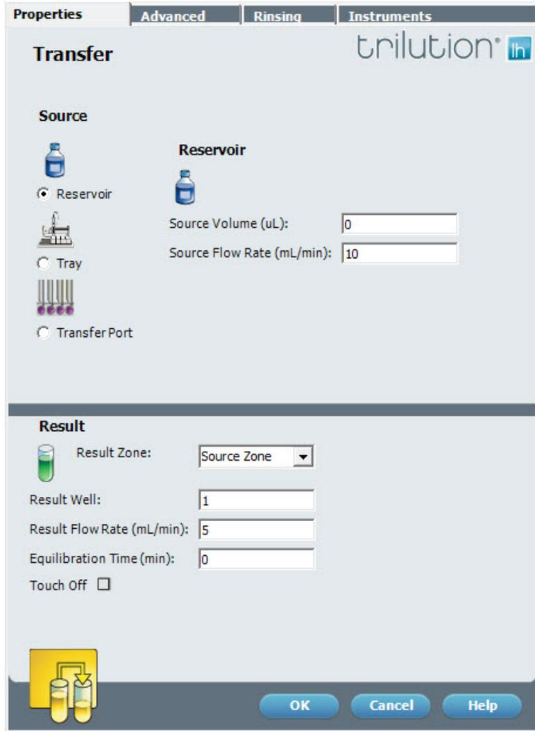
The screenshot displays the 'Transfer' dialog box in the Trilution LH software. The dialog has four tabs: 'Properties', 'Advanced', 'Rinsing', and 'Instruments'. The 'Properties' tab is active, showing the following settings:
