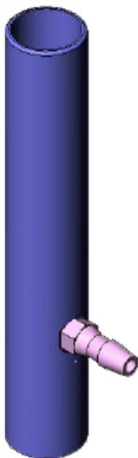
Drain/Rinse Station for Inside Rinse of Probe
