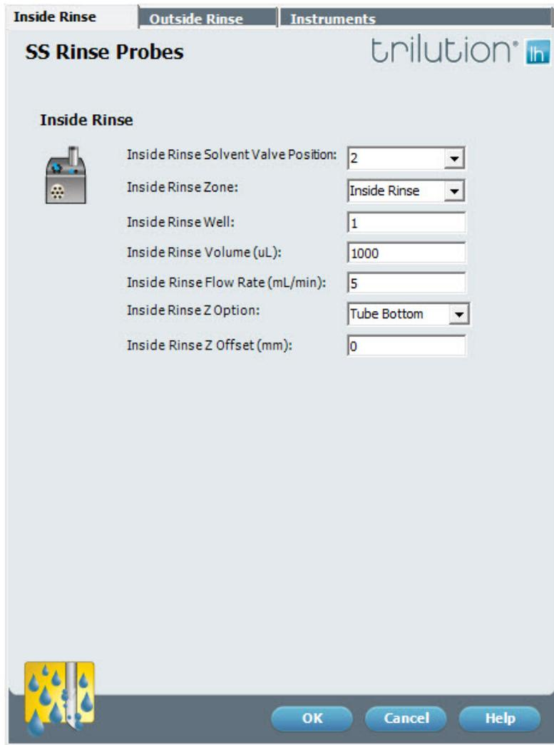
The screenshot shows the 'SS Rinse Probes' dialog box with the 'Inside Rinse' tab selected. The 'trilution' logo is in the top right corner. The 'Inside Rinse' section includes a small icon of a probe and the following settings:
