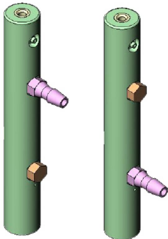
Rinse Station for Outside Rinse of Probe (Static)
